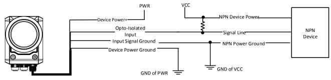
Figure 6-9 Input Signal Connecting to NPN Device
