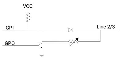
Figure 6-5 Internal Circuit of Bi-Directional Signal
