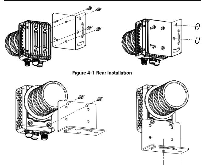
Figure 4-2 Front Installation
