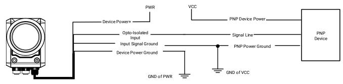
Figure 6-8 Input Signal Connecting to PNP Device
