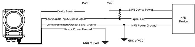
Figure 6-13 Input Signal Connecting to NPN Device
