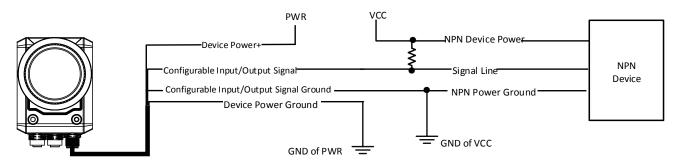
Figure 6-15 Output Signal Connecting to NPN Device
