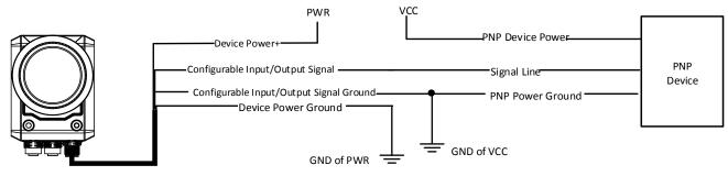
Figure 6-14 Output Signal Connecting to PNP Device
