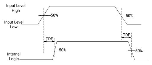
Figure 6-6 Input Logic Level
