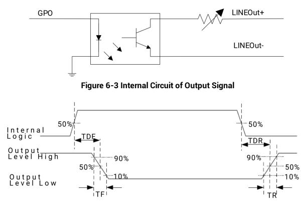
Figure 6-4 Output Logic Level
