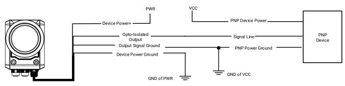
Figure 6-10 Output Signal Connecting to PNP Device
