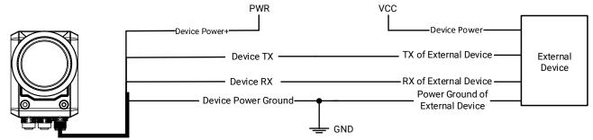
Figure 6-18 RS-232 Serial Port Wiring
