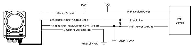
Figure 6-12 Input Signal Connecting to PNP Device
