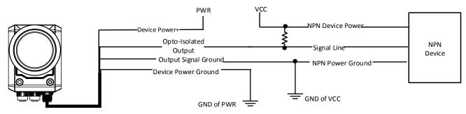
Figure 6-11 Output Signal Connecting to NPN Device
