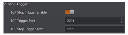
Figure 8-31 Stop Trigger via TCP
