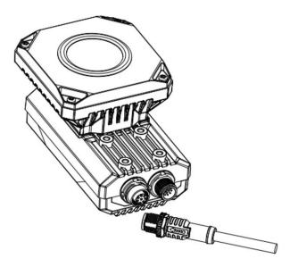
Figure 5-3 Gigabit Ethernet Interface Wiring
