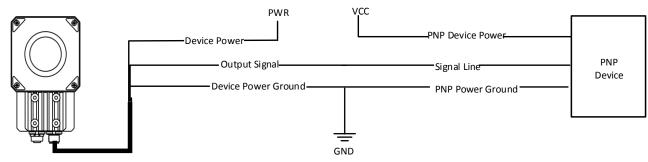
Figure 4-5 Output Signal Connecting to PNP Device
