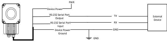
Figure 4-9 RS-232 Serial Port Wiring
