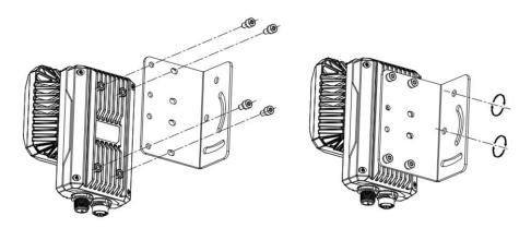
Figure 5-1 Rear Installation
