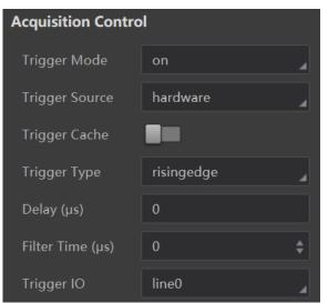
Figure 8-7 Set and Execute Hardware Trigger Mode
