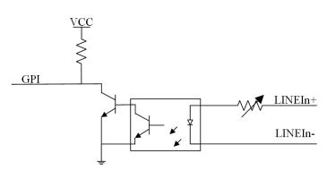
Figure 4-1 Internal Circuit of Input Signal
