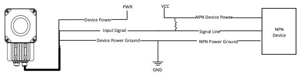
Figure 4-4 Input Signal Connecting to NPN Device
