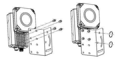
Figure 5-2 Front Installation
