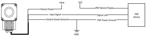
Figure 4-3 Input Signal Connecting to PNP Device
