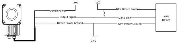
Figure 4-6 Output Signal Connecting to NPN Device
